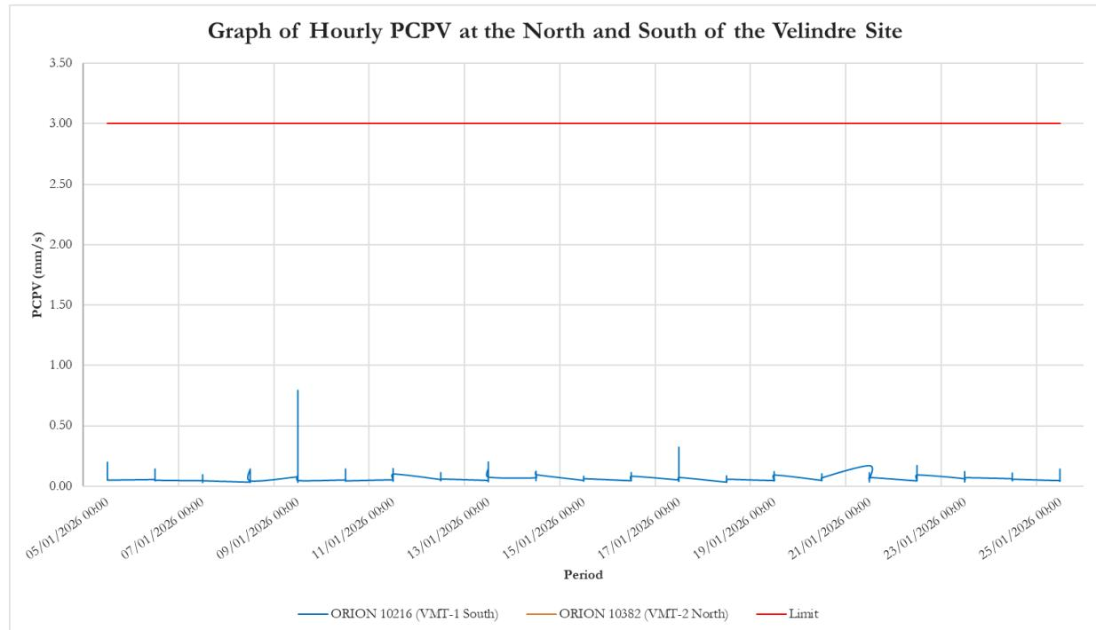
**No vibration data recorded exceeded the 1.00mm/s limit at the South monitoring station on the Velindre site in the period 05/01/26 – 25/01/26. No data recorded for the North monitoring station due to signal issues.**
