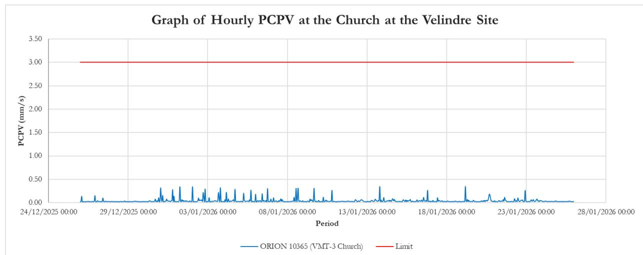
**No vibration data recorded exceeded the 1.00mm/s limit at the Church monitoring station outside the Velindre site for the period covering 26/12/25 – 25/01/26.**
